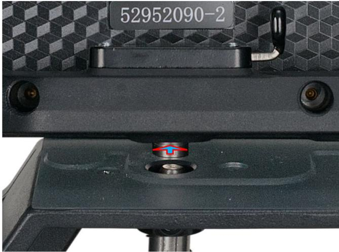
Align the vertical positional posts with their corresponding alignment holes and insert them.
