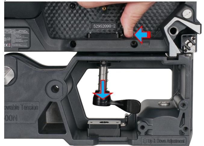
To unlock the vertical connector, rotate lever to the right (counter-clockwise), then press spring-loaded locking latch inward. The vertical connector will spring-drop open.
