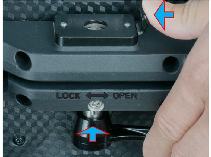
Press the spring-loaded locking latch toward the left while pressing vertical connector up into locking-latch.
