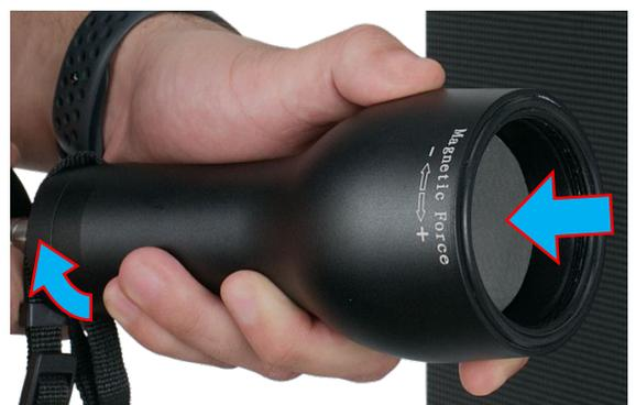
The perceived “Magnetic Force” is relative to the distance the magnet is from the surface. Turning the knob clockwise, in the “+” direction, advances the magnet, moving it closer to the front, and turning it counterclockwise, in the “-” direction, retracts the magnet, moving it away from the front.
